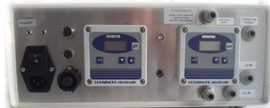
Back of the operating- and display-element with connectors for instrumentation and air supply
